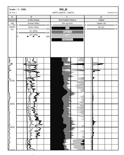
Figure 2: In-situ stress regimeand a safe mud weight window analysis obtained using poro-elastic based method.
